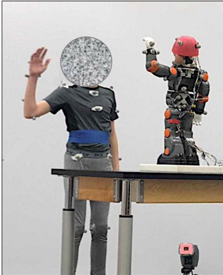
Figure 1. Participant interacting with Zeno the robot, instrumented with markers on the head, arms, and torso.
